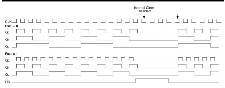
The EN signal will freeze the internal clocks to the flip-flops on the first falling edge of CLK after its assertion. The internal dividers will maintain their state during the internal clock freeze and will return to clocking once the internal clocks are unfrozen. The outputs will transition to their next states in the same manner, time and relationship as they would have had the EN signal not been asserted.
